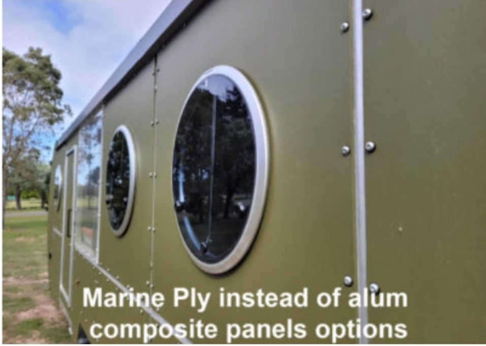
5. Marine Ply instead of alum composite panels option
